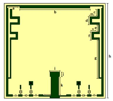
$\begin{array}{l} a{=}3.25mm,b{=}18mm,c{=}2mm,d{=}2mm,e{=}2mm,f{=}2mm,g{=}\\ 9.75mm,h{=}24mm,i{=}2.5mm,j{=}1.25mm,k{=}5mm,l{=}2.25mm\\ m{=}2mm.n{=}1.75mm \end{array}$
