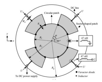
Fig 2.2.9 Circular Monopolar Patch Antenna
