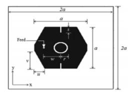
Fig 2.2.4 Polygon-Shaped Slotted Dual-Band Antenna
