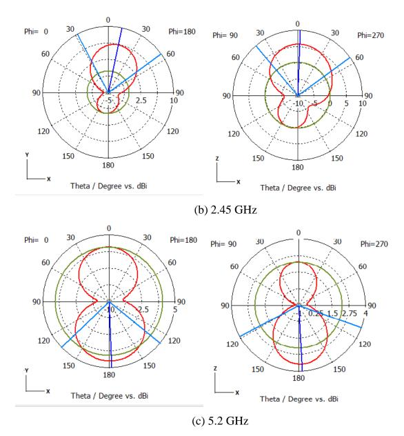
Fig 4.2.1:Radiation characteristics of the proposed antenna
