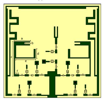
$a\!=\!4.25 mm, b\!=\!1.5 mm, c\!=\!9.25 mm, d\!=\!2.5 mm, e\!=\!5.5 mm, f\!=\!1.15 mm$
