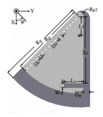
Fig 2.2.1 Compact Dual Band Antenna for WBAN application
