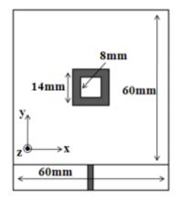
Fig 2.2.13 Wearable Antenna for WLAN Band Applications
