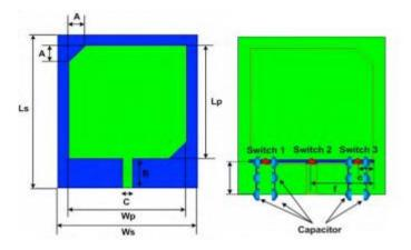
Fig 2.2.15 Reconfigurable circularly polarized textile antenna
