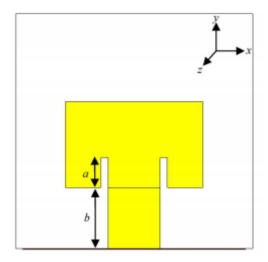
Fig 2.2.8 Frequency-Reconfigurable Microstrip Patch-Slot Antenna
