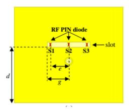
Fig 2.2.11 Frequency Reconfigurable Microstrip Patch Antenna with switches S1,S2& S3
