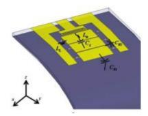
Fig 2.2.7 Zeroth-order resonant antenna
