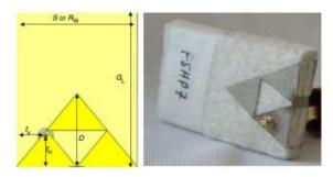
Fig 2.2.3 Dual-band Planar inverted-F antenna
