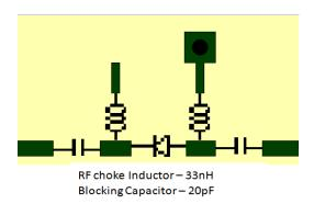
Fig.3.3.1: Biasing circuit
