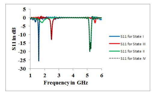
Fig.4.1.2 Simulated reflection characteristics across different operating states
