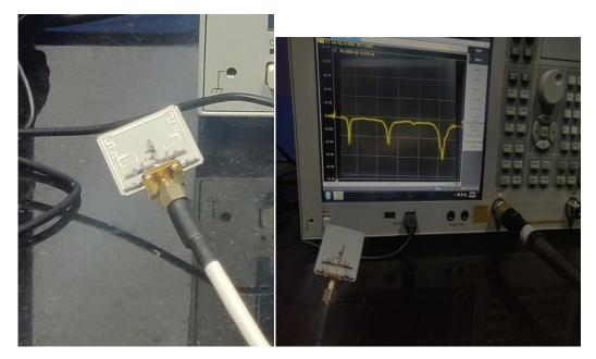
Fig.4.4.2: Free space Measurement of Reflection Characteristics
