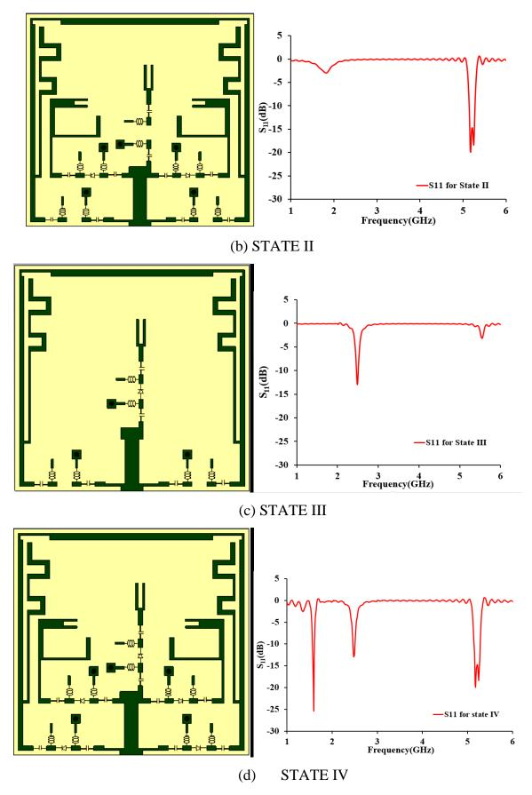
Fig.4.1.1: Simulated reflection characteristics of the proposed antenna
