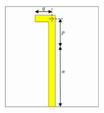
Fig 2.2.10 Narrowband Microstrip Slot Antenna
