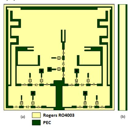
Fig.3.1.1: Design of the Proposed Antenna (a) Front View (b) Side View
