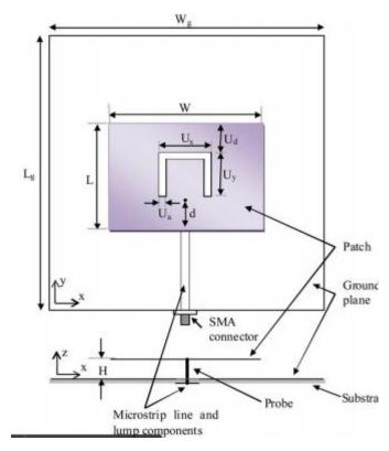
Fig 2.2.12 Frequency tunable U-slot microstrip patch antenna
