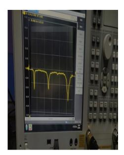
Fig.4.4.3: On-Body (wrist) Measurement of Reflection Characteristics
