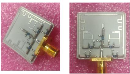
Fig.4.4.1: Fabricated prototype of the antenna
